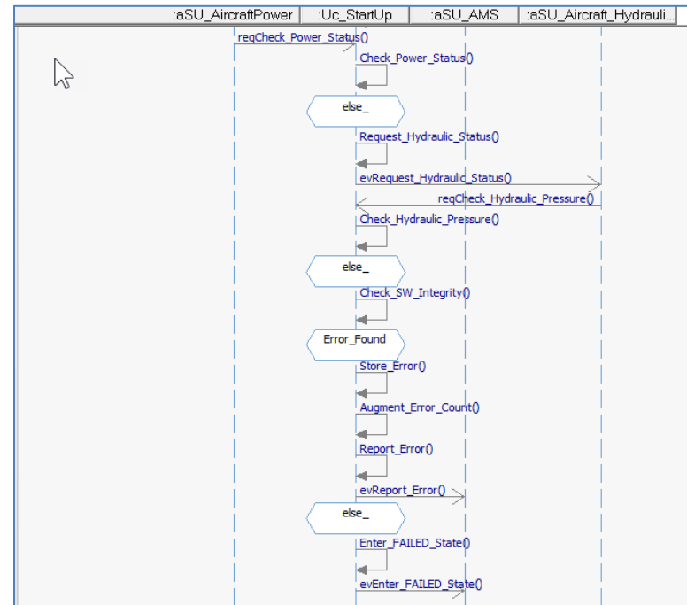
Figure 68: Scenario multiple errors (part 2)
