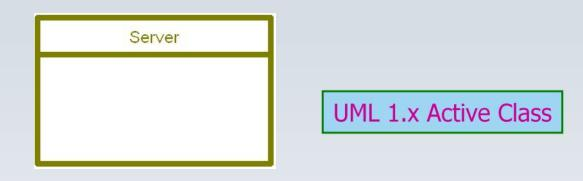
In UML 2.0 the notation has changed to double vertical lines
